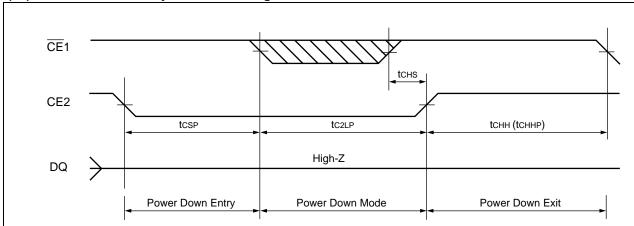
Note: This Power Down mode can be also used as a reset timing if "POWER-UP timing" above could not be satisfied and Power Down program was not performed prior to this reset.
