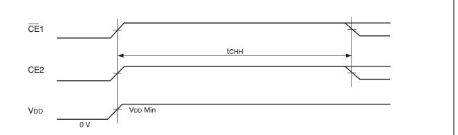
Note: The tchh specifies after Vdd reaches specified minimum level and applicable both  $\overline{\text{CE}}1$  and CE2. If transition time of Vdd (from 0 V to Vdd Min) is longer than 50 ms, POWER-UP Timing #1 must be applied.
